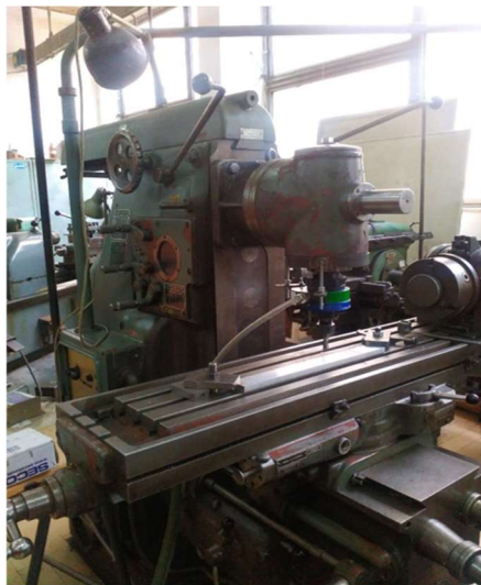
Figure 1. Universal milling machine „Prvomajska“ UGH with solid carbide end mill
